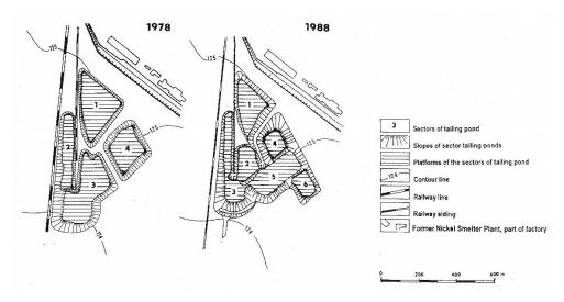
Figure 4. Landfill sludge fields development between 1978–1988.
